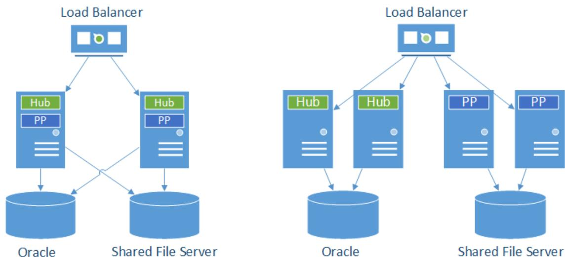
High-availability configuration that deploys Pipeline Pilot and Foundation Hub instances on shared servers or separate nodes.
